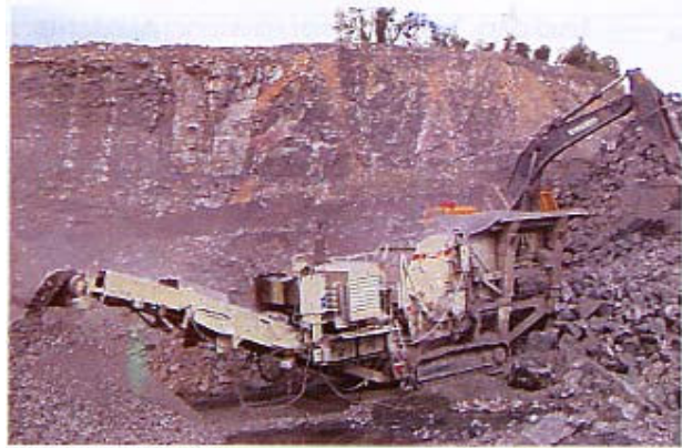
A Nordberg LT1415 Lokotrak forms part of Roadstone Dublin's recycling plant
